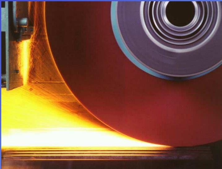
**Grind hardening** utilizes the dissipated heat in grinding in order to induce martensitic phase transformations in the surface layers of the processed components.
