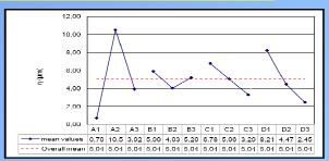
Implementation of ANOM and ANOVA analyses for calculation of the optimum value of each factor, and their responsibility (%) on average surface roughness (µm)
