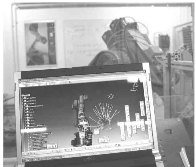
Figure 7 – Scanning simulation in Catia environment
