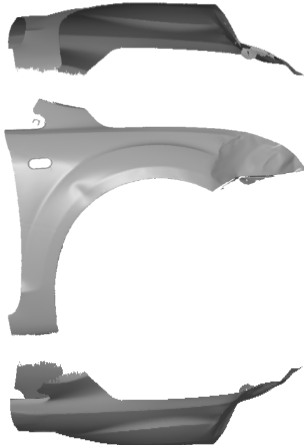
Figure 9 – 3D fender model scanned using the described method
