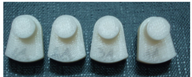
Figure 9 – Form Error on RP cylindrical features
