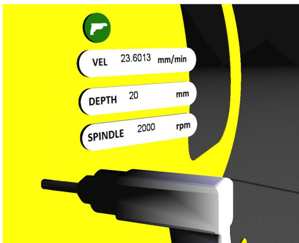
Figure 15 – Drilling test-case, executed on a virtual aircraft fuselage.
