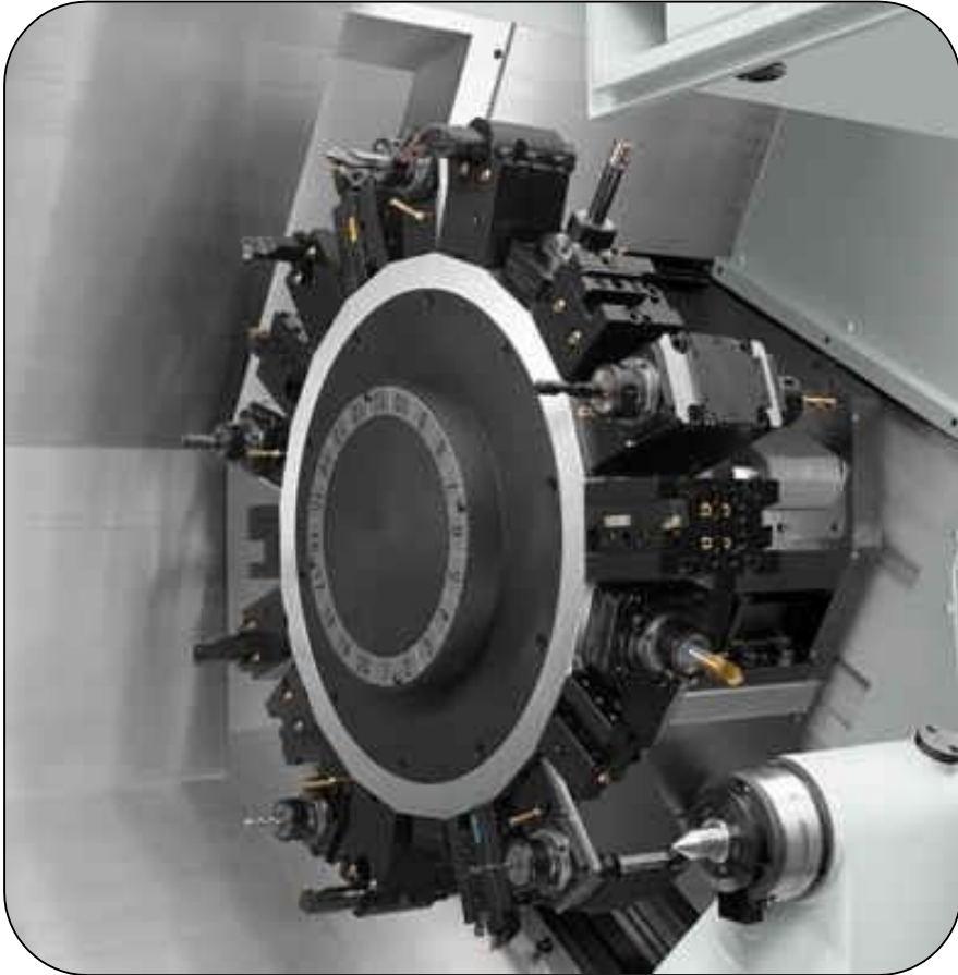
Figure 9:CNC lathe tool turret
