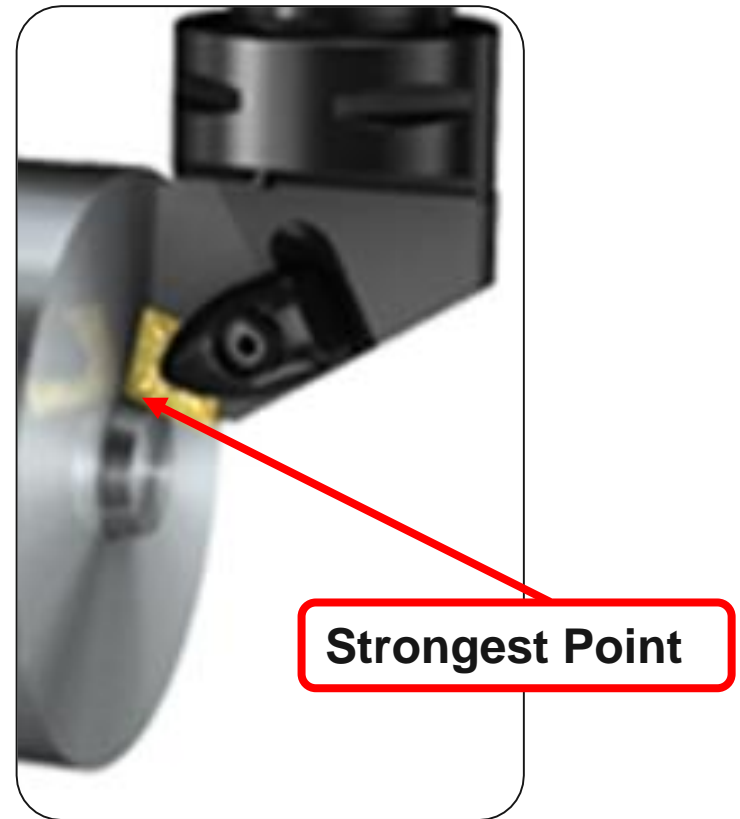
Figure 3-16: The effect of the lead angle on the strength of the insert. Increasing the lead angle will greatly reduce tool breakage when roughing or cutting interrupted faces
