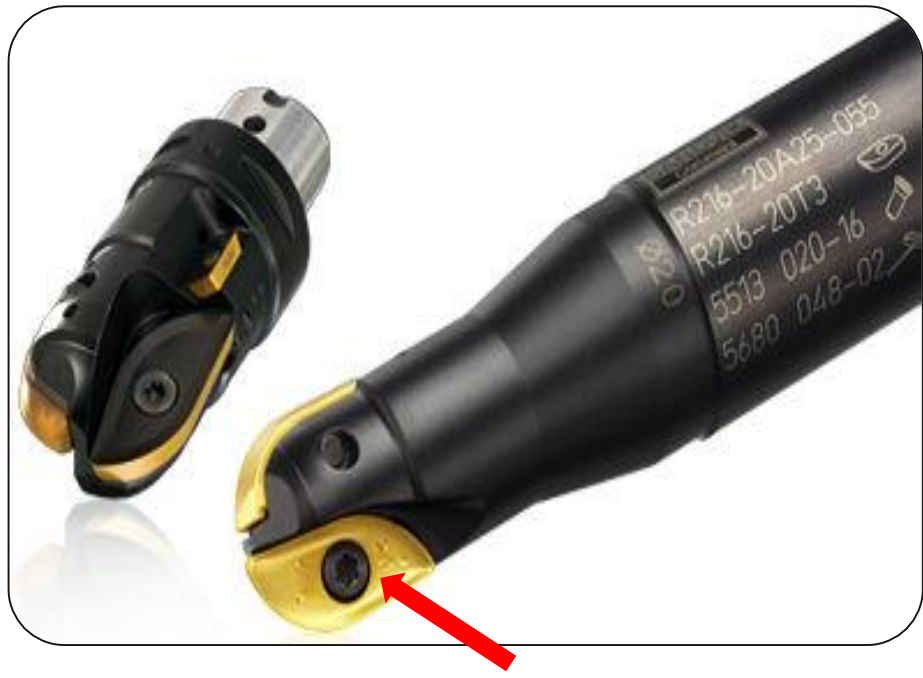
Figure 3-23: Ball nose end mills featuring Inserts with two cutting edges (Photo SANDVIK Coromant)
