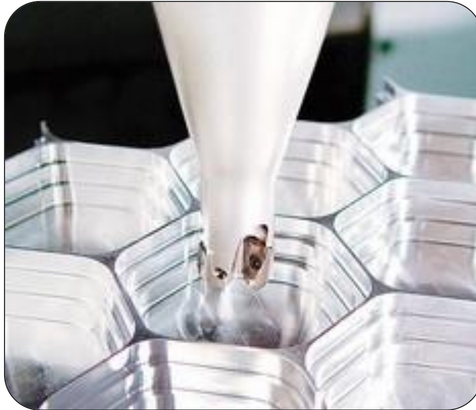
Figure 3-40 :Indexable Inserted end mill suitable for multi-functional milling
