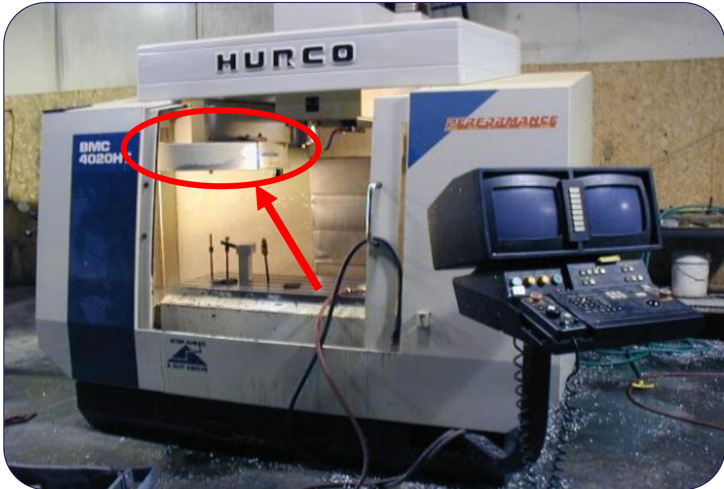
FIGURE 4-20: A vertical spindle machining center using carousel tool storage (Photo courtesy of HURCO)
