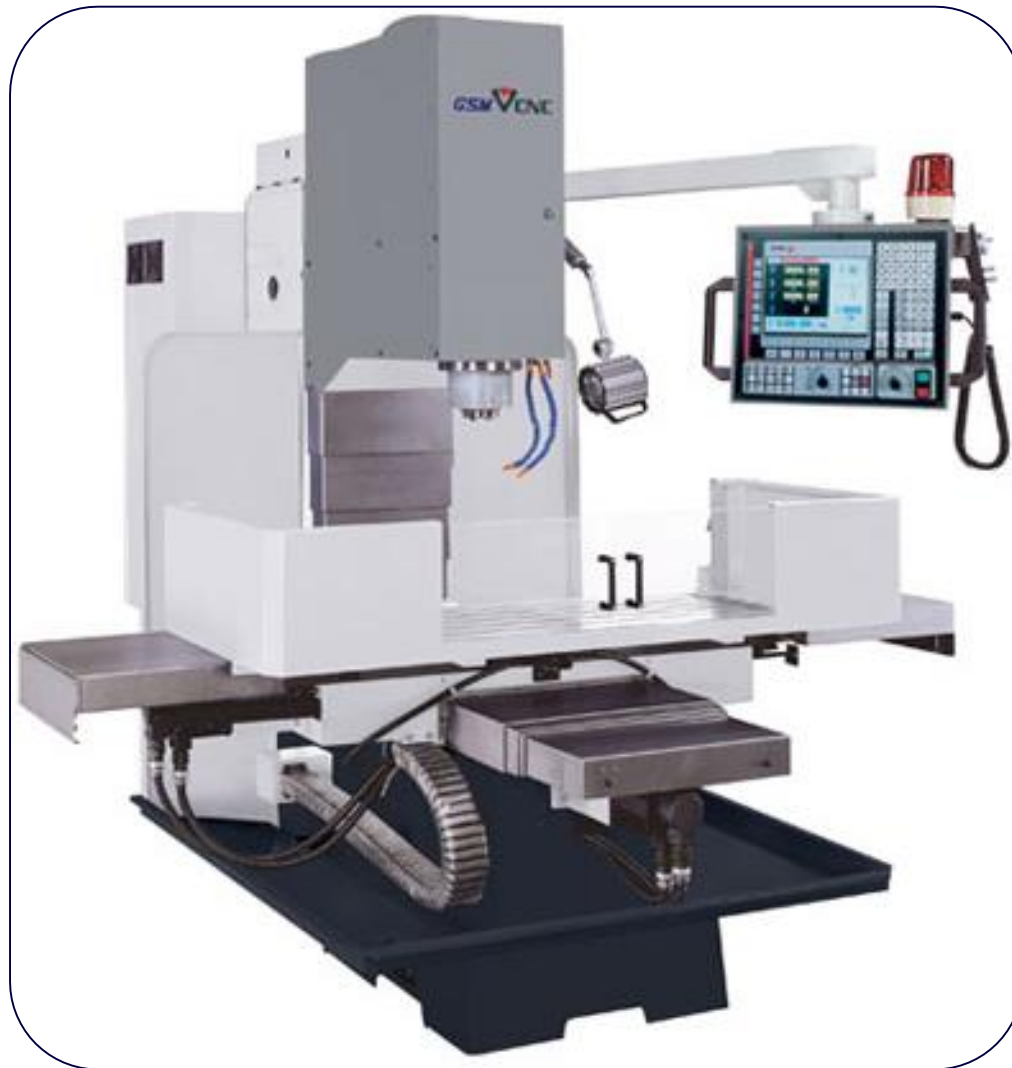
FIGURE 4-1: A vertical spindle CNC milling machine (Photo courtesy of GSM CNC CO.)
