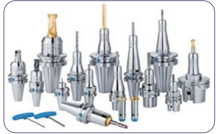
FIGURE 4-11 An assortment of tools and toolholders used with CNC machining center
